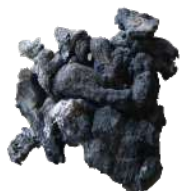
Coal clinker reduce efficiency of combustion
